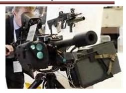
**Short Description:** The HV ABMS consists of a Fire Control System, an Ammunition Programmer and XX x XX mm Air Burst Munitions. High explosive, Flash and Bang, Counter defilade, increased lethality, improved accuracy.
